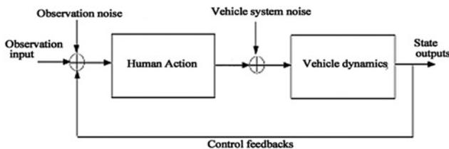
Fig. 2 Structure of a DVU model [1]
