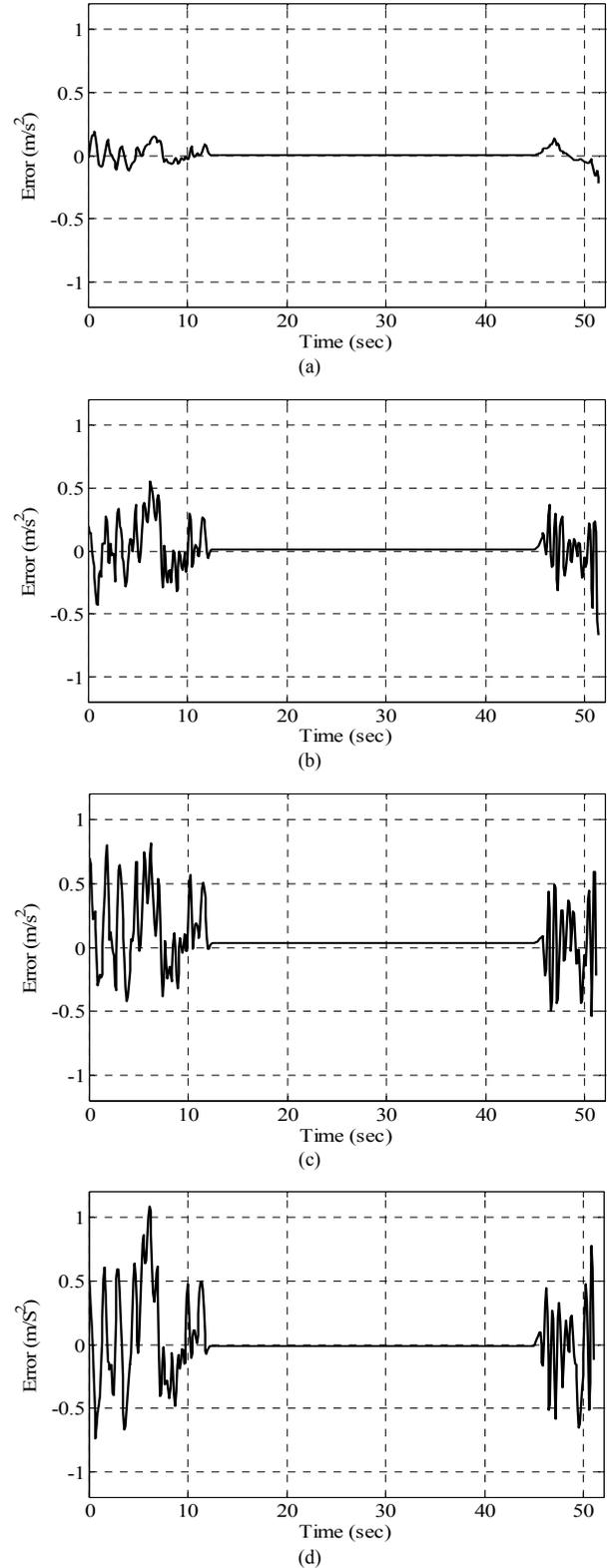
Fig. 7. Comparison of errors for the same test vehicles of Fig. 6, (a) 0.1 second ahead model, (b) 0.2 second ahead model, (c) 0.3 second ahead model, (d) 0.5 second ahead model.
