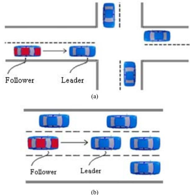
Fig. 1. Examples of situations that a Stop&Go maneuver may occur, (a) An intersection with traffic light, (b) Congested road.
