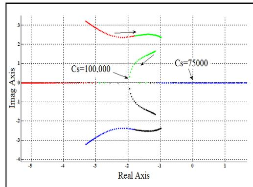
Figure 6. The effect of  $C_2$  variation on directional stability
