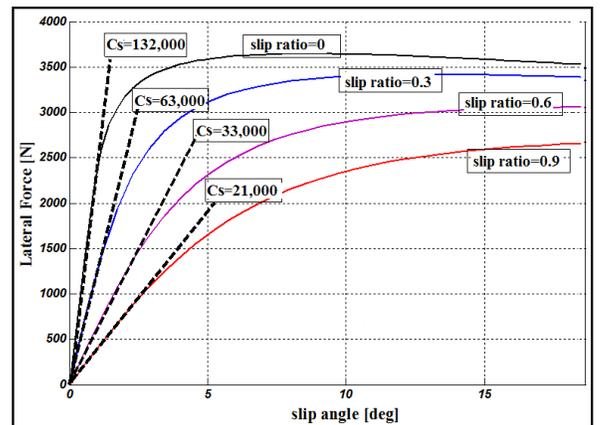
Figure 3. Cornering stiffness dependency with wheel slip ratio
