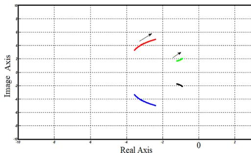
Figure 4. The effect of  $C_1$  variation on directional stability
