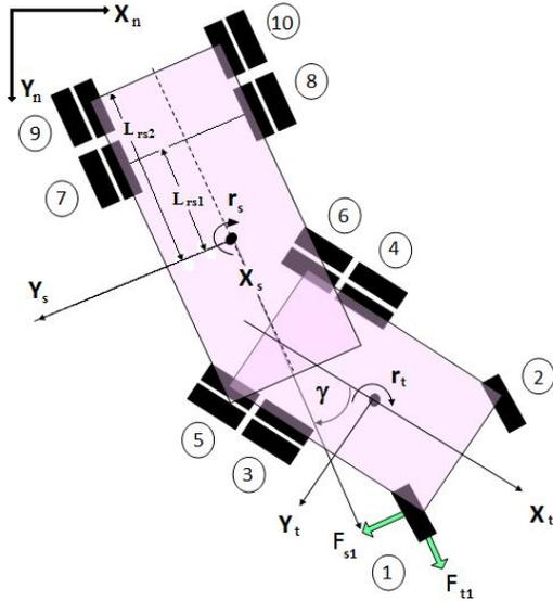
Figure 1. Fourteen degrees of freedom articulated vehicle model
