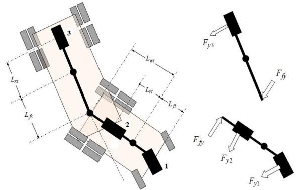
Figure 2. Linear model of the articulated vehicle
