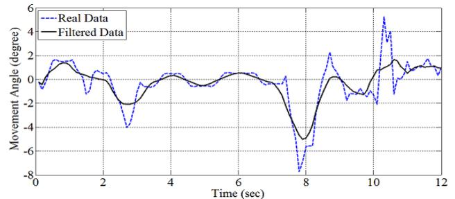
Fig. 4. Comparison of unfiltered and filtered data: Movement Angle.
