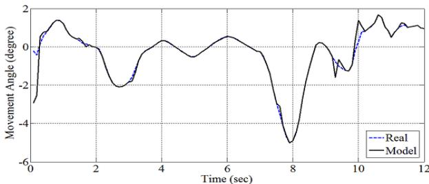
Fig. 7. Comparison of the ANFIS model and real data: Movement Angle.
