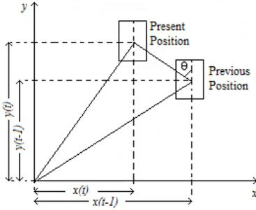
Fig. 5. The movement angle of the overtaker vehicle.
